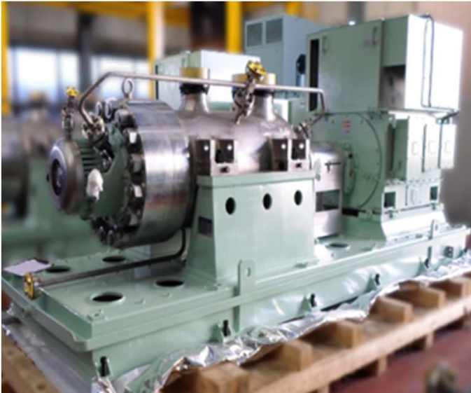
Safety Injection Pump
