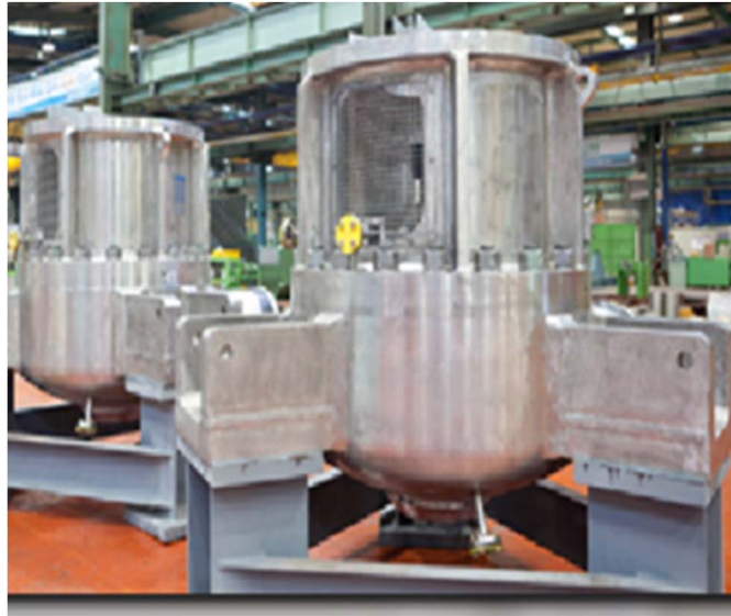
Shutdown Cooling Pump
